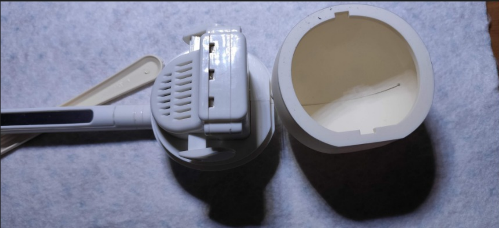
Opening the head requires the silicone front to be detached. Note: this image was produced after the instrument was reassembled due to me forgetting to take it earlier.
