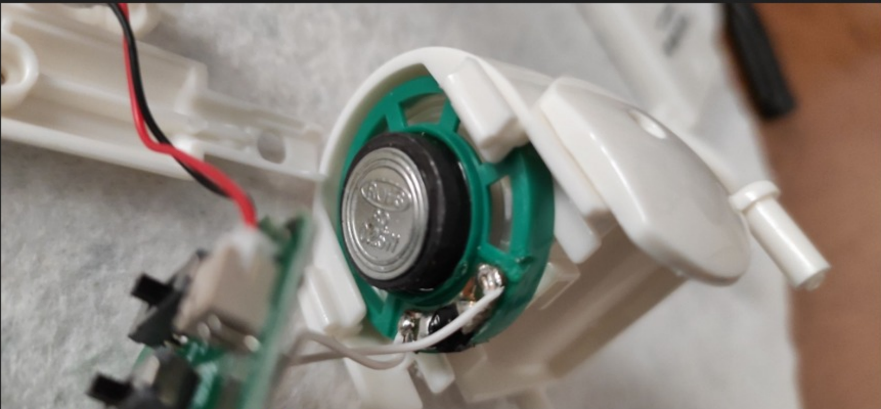
The speaker is a standard 8Ω, 0.25W one.
