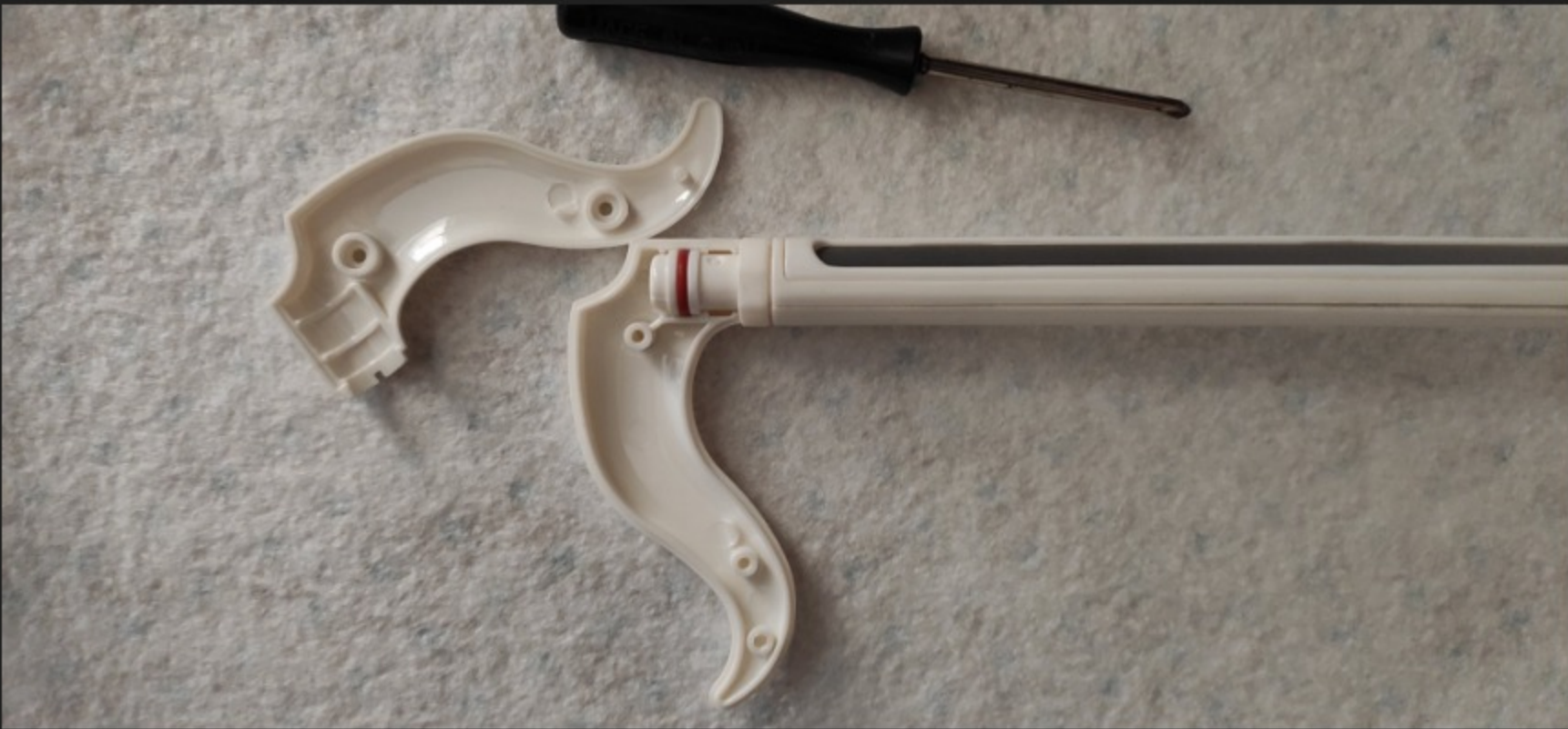
Opening the tail shows that the end of the neck is held together by a plastic ring and a red rubber band.
