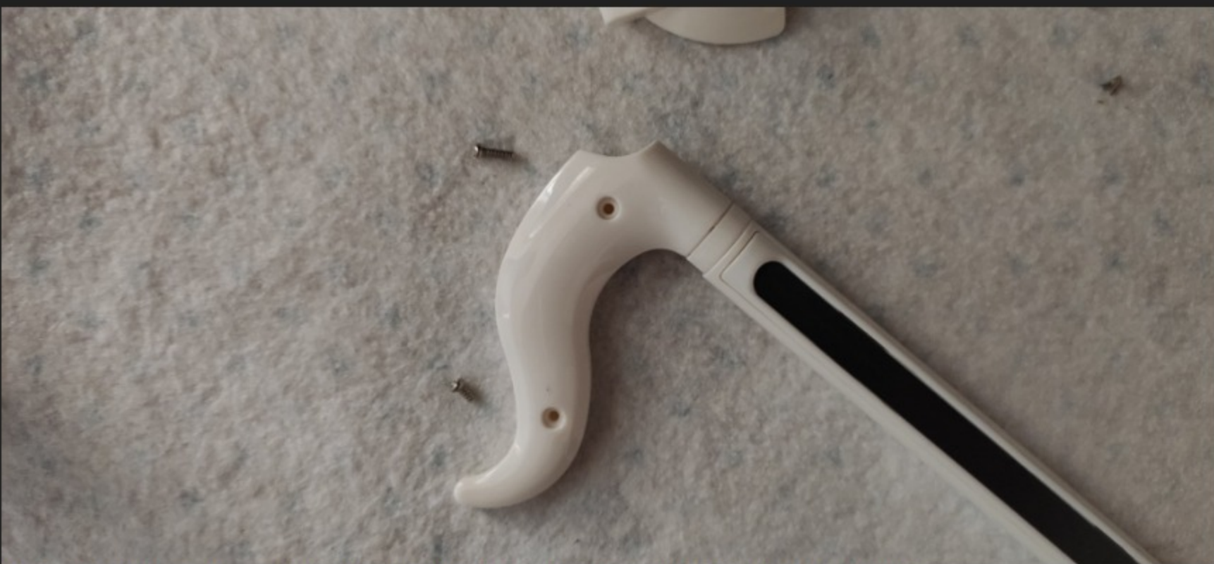
All screws used are the same length, except for that at the very end of the Otamatone's tail.
